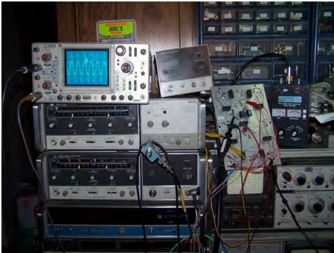
Figure 24: Switching Unit Test Setup consisting of just the MFJ-259 and dual trace oscilloscope (The other equipment is not used for this test)
