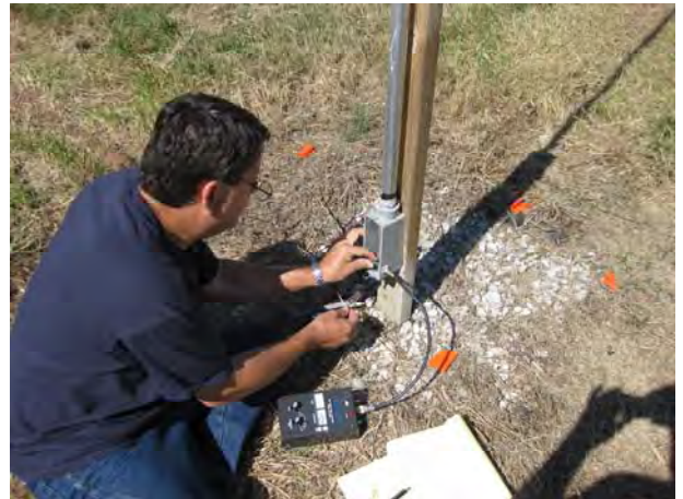
Figure 20: W5ZN Measuring Self-resonance of Vertical Elements
